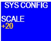
The **Brake Scale** screen allows the driver to adjust the brake levels. The **Brake Scale** number represents the level of trailer braking that the DireLink will apply to the trailer brakes when the tow-vehicle brakes are applied. The value can be adjusted from +1 to +20 with +1 being very light braking and +20 being very heavy braking. (The default level is set at +3.)
