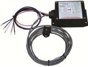
The TSC continuously monitors trailer sway and rapidly identifies a trailer sway condition. When sway exceeds a safe level the TSC quickly intervenes by applying the electric brakes, on the correct side of the trailer with the proper braking level, to bring the trailer sway under control without any intervention by the driver.
